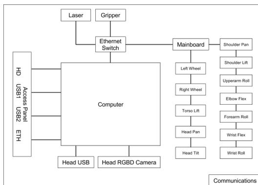
Figure 4: Routing diagram of communications buses within the Fetch mobile manipulator. Shown are the RS-485, Ethernet, and USB connections.
